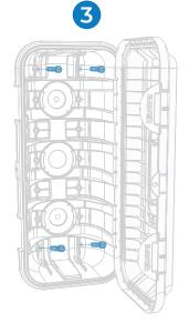
FIX THE FIRECAB ON THE SELECTED SURFACE BY CHOOSING APPROPRIATE FASTENERS ACCORDING TO WALL MATERIAL AND TOTAL WEIGHT
