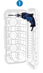
DRILL HOLES, **AT LEAST 2 PER SIDE**, ON TOP AND BOTTOM OF THE BLACK FRAME
